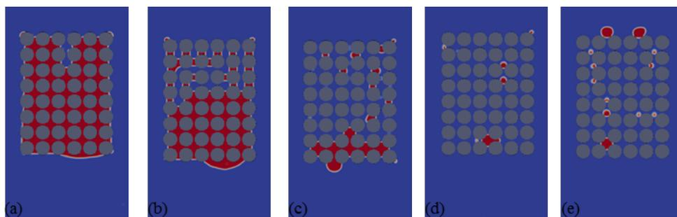
**Figure 3.** Numerical results after drainage (kinematic viscosity  $3.14 \times 10^{-8}$  m<sup>2</sup>·s<sup>-1</sup>; surface tension 0.032 N/m) for different contact angle: (a) 30°, (b) 60°, (c) 90°, (d) 120° and (e) 150°.
