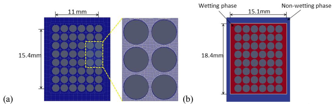
Figure 2: The computational domain: (a) The granular obstacles are arranged in regular array (25×45.7 mm<sup>2</sup>; 48 obstacles; particle diameter of 2 mm and throat size of 200  $\mu$ m). (b) The non-wetting phase (blue) and wetting phase (red).
