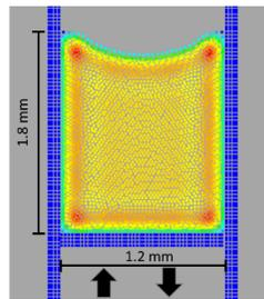
**Figure 3. Capillary tube with a moving substrate.**
