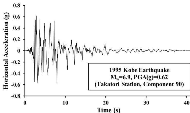
Figure 2. Input acceleration time-history of the 1995 Kobe earthquake
