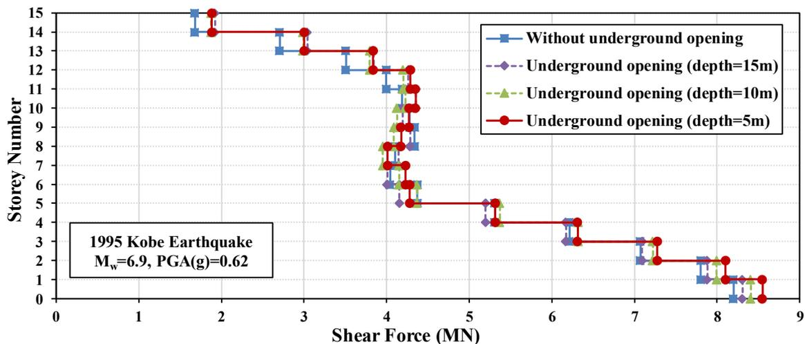
**Figure 4. The distribution of maximum shear force in the building subjected to the 1995 Kobe earthquake considering different underground opening arrangements**
