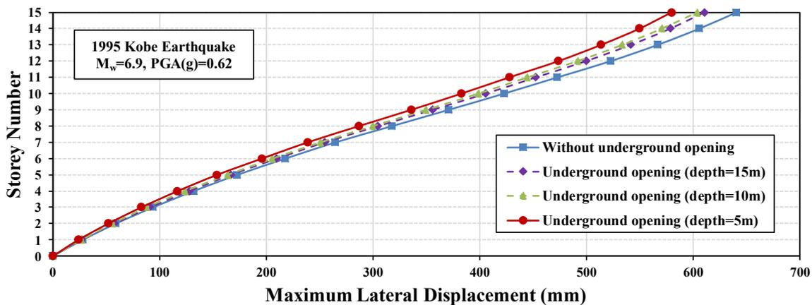
**Figure 6. Maximum lateral displacement of the building subjected to the 1995 Kobe earthquake considering different underground opening arrangements**
