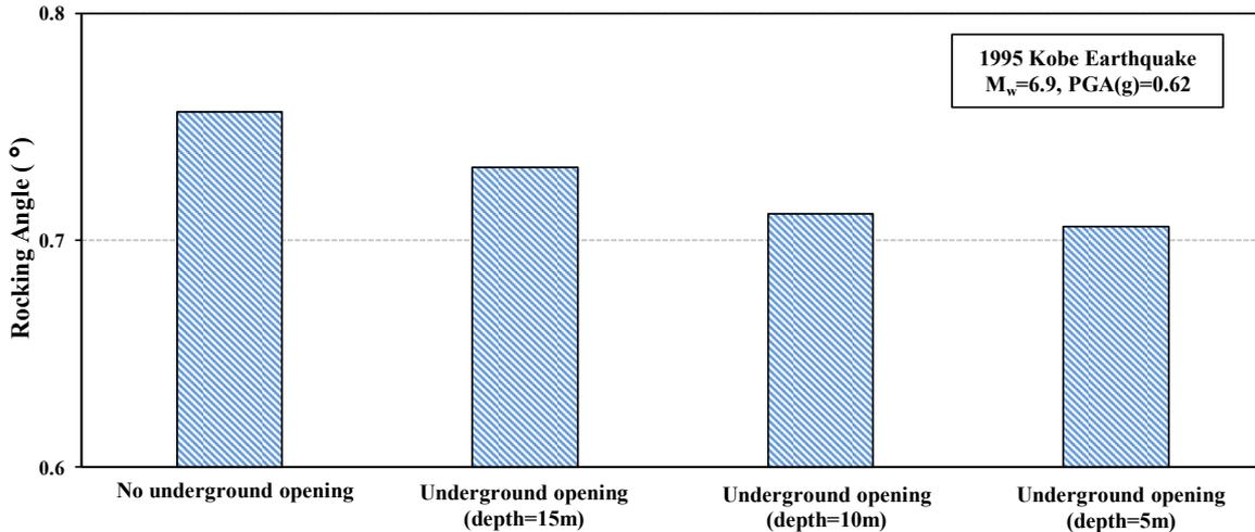
**Figure 3. Maximum foundation rocking angle subjected to the 1995 Kobe earthquake considering different underground opening arrangements**
