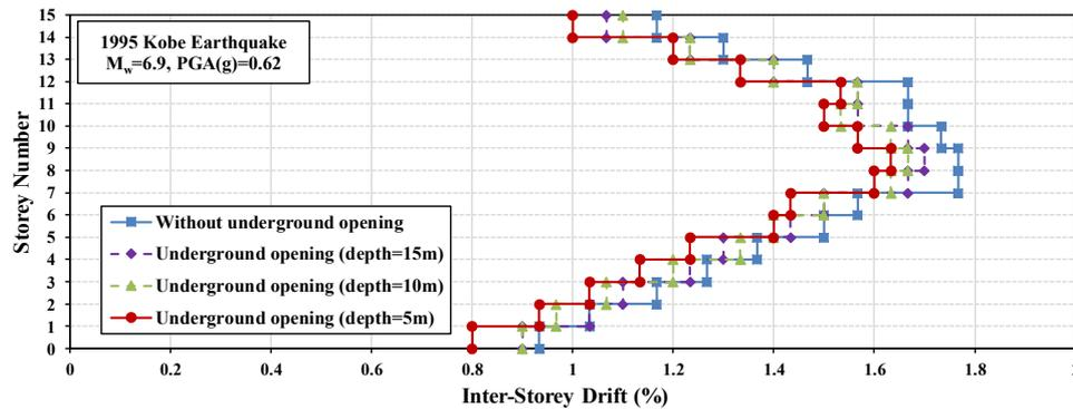
**Figure 7. Maximum inter-storey drifts of the building subjected to the 1995 Kobe earthquake considering different underground opening arrangements**
