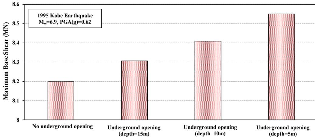
**Figure 5. Maximum base shear in the building subjected to the 1995 Kobe earthquake considering different underground opening arrangements**
